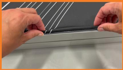
4 After the corners and centers of each panel are inserted, work your way around the perimeter of the frame starting from the middle and working your way out, pushing the silicone edge in securely.
