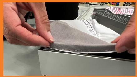
Once all four corners are in place, push the silicone bead into the middle of each frame side.
