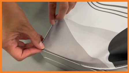
2 To insert the SEG edge, use your thumb and forefinger to tuck the silicone edge and press it into the frame channel. The stitching should be fully inserted into the channel and will not show.
