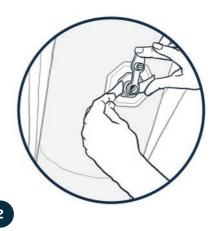
Open the deflation valve by pulling on the valve lid. Immediately the strut will start to deflate. Afterwards the Counter can be stowed in the transport bag.
