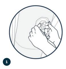
Open the velcro strap to access the valve plug.
