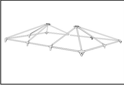
Install the crown cluster bracket by inserting a hip pole first - and then inserting one pole at a time, clockwise around the bracket. It may be necessary to lift up on the cluster to get the poles installed and locked into place. Repeat for the second crown cluster bracket.
