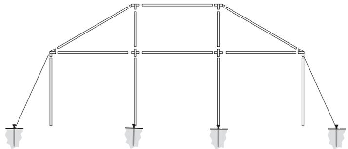
36" Stake driven within 6" from the top of the ground straight down or a maximum 10 degree angle
