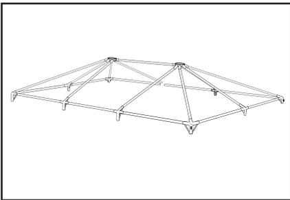
Install the ridge rafter pole between the two crown cluster brackets. Ensure that both snap pins lock into place at both ends of the pole.
