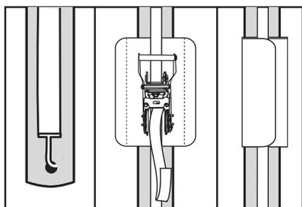
As with the tent top straps, the intermediate tent top straps will also be attached to the 7' leg poles by inserting the hook into the hole at the bottom of the poles. Locate the ratchet in the middle of the strap and tighten until the strap is taut enough to secure the canopy.
