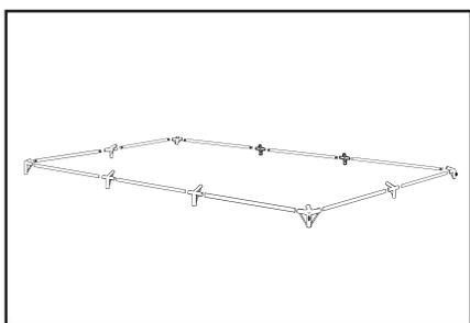
Lay out the erection site by first placing the corner brackets, intermediate brackets and perimeter poles in sequence per the diagram to the left for assembly. Do not install legs or roof rafters at this time.
