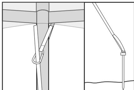
Locate the remaining 4 outguy straps. Connect the carabiner at the top of the strap to the intermediate bracket by looping the carabiner around the bracket and clipping it back on itself. Locate the 3' ground stakes and wrap the looped strap (found at the bottom end of the outguy straps) around the head of the stake twice. Drive the stakes into the ground 5' out from each corner leg and ratchet the strap until it is taut. Repeat this step on the 3 remaining intermediate legs.
