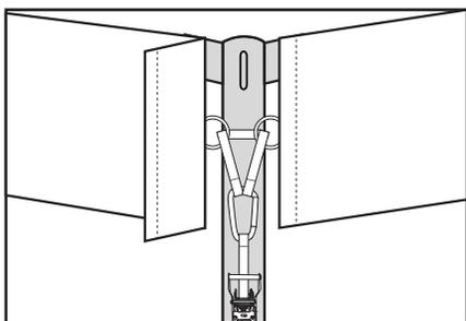
Attach tent top to the frame with the tent top straps. Bring the "Y" straps (located at the very top of the tent top straps) through the metal rings on each of the tent top valances and secure the looped ends of the "Y" straps into the carabiner. Fold the valance flap over the "Y" straps where the strips of velcro line up to finish the corner. Repeat this step at the remaining three corners. **\*\*Do not hook carabiner directly to metal valance rings!\*\***
