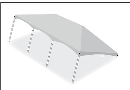
Lift one of the 30' sides of the frame and install the legs along that side. Install the corner legs before the intermediate legs.
