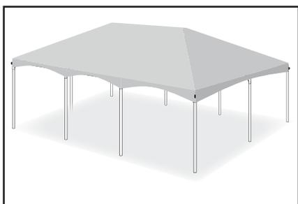
Finish by installing the legs in the final two intermediate brackets on the 20' sides. Make sure all snap pins are locked in place.
