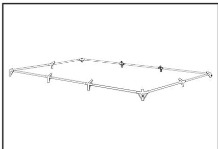
Begin assembly of the frame by inserting the perimeter poles into the corner brackets and ensure that the snap pins lock into place. Next, move to the intermediate bracket and repeat the procedure. Continue this process until the perimeter framework is assembled.
