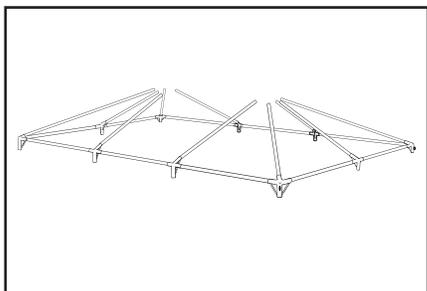
Insert hip poles into corner brackets at all four corners. Insert the intermediate poles into the intermediate brackets at all six center points. All ten poles should be installed with the open hole end towards the sky and the snap pin ends towards the ground. Ensure that all snap pins lock into place in all brackets.
