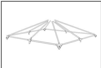
Insert hip poles into corner brackets at all four corners. Insert the intermediate poles into the intermediate brackets at all four center points. All eight poles should be installed with the open hole end towards the sky and the snap pin ends towards the ground. Ensure that all snap pins lock into place in all brackets.
