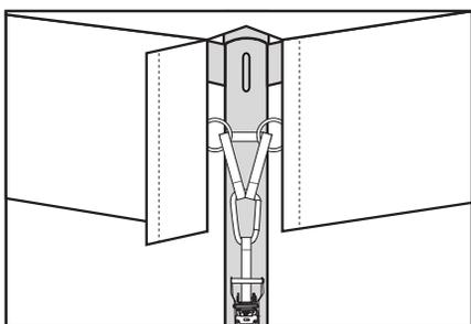
Attach tent top to the frame with the tent top straps. Bring the “Y” straps (located at the very top of the tent top straps) through the metal rings on each of the tent top valances and secure the looped ends of the “Y” straps into the carabiner. Fold the valance flap over the “Y” straps where the strips of velcro line up to finish the corner. Repeat this step at the remaining 3 corners. **\*\*Do not hook carabiner directly to metal valance rings!\*\***
