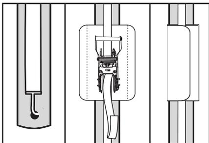
Attach the bottom of the tent top straps to the legs of the tent by inserting the hook into the hole at the bottom of the leg poles. Locate the ratchet in the middle of the strap and tighten until the strap is taut enough to secure the canopy. Repeat this step at the remaining 3 corner legs.
