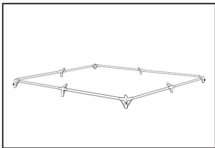
Begin assembly of the frame by inserting the perimeter poles into the corner brackets and ensure that the snap pins lock into place. Next, move to the intermediate bracket and repeat the procedure. Continue this process until the perimeter framework is assembled.
