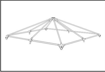
Install the crown cluster bracket by inserting a hip pole first - and then inserting one pole at a time, clockwise around the bracket. It may be necessary to lift up on the cluster to get the poles installed and locked into place.
