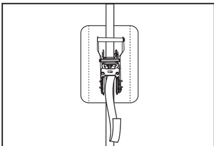
Once all stakes have been secured and straps ratcheted taut, fold all extra outguy strap length into the white vinyl covers with velcro closure.
