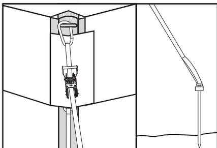
Locate the outguy straps and connect the carabiner at the top of the strap to the cast eyelet that is on the outside of each of the corner brackets. Locate the 3' ground stakes and wrap the looped strap (found at the bottom end of the outguy straps) around the head of the stake twice. Drive the stakes into the ground 5' out from each corner leg and ratchet the strap until it is taut. Repeat this step on the three remaining corner legs.
