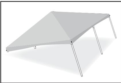
Lift one side of the frame and install the legs along that side. Install the corner legs before the intermediate legs.
