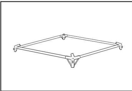
Begin assembly of the frame by inserting the perimeter poles into the corner brackets and ensure that the snap pins lock into place. Continue this process until the perimeter framework is assembled.
