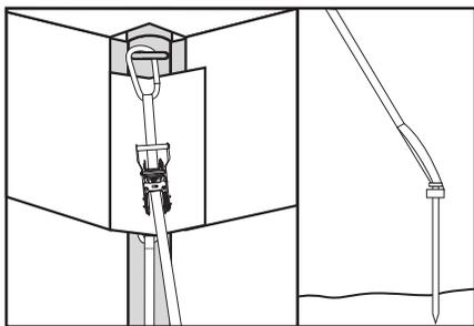
Locate the outguy straps and connect the carabiner at the top of the strap to the cast eyelet that is on the outside of each of the corner brackets. Locate the 3’ ground stakes and wrap the looped strap (found at the bottom end of the outguy straps) around the head of the stake twice. Drive the stakes into the ground 5’ out from each corner leg and ratchet the strap until it is taut. Repeat this step on the three remaining corner legs.
