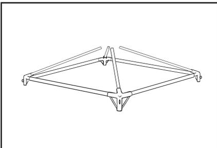
Insert hip poles into corner brackets at all four corners. All four poles should be installed with the open hole end towards the sky and the snap pin ends towards the ground. Ensure that all snap pins lock into place in all brackets.
