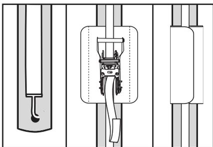
Attach the bottom of the tent top straps to the legs of the tent by inserting the hook into the hole at the bottom of the leg poles. Locate the ratchet in the middle of the strap and tighten until the strap is taut enough to secure the canopy. Repeat this step at the remaining 3 corner legs.
