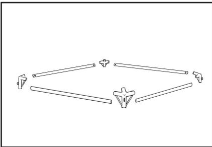
Lay out the erection site by first placing the corner brackets and perimeter poles in sequence per the diagram to the left for assembly. Do not install legs or roof rafters at this time.
