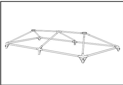
Insert both ridge rafter poles into the crown cluster and the roof rafter brackets to complete the roof structure. Ensure that all snap pins lock into place in all brackets.
