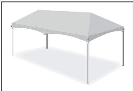
Lift the opposite 10' side of the tent and insert the legs into the brackets as in the previous step. This will complete installation of the four corner legs. Make sure all snap pins are locked in place.
