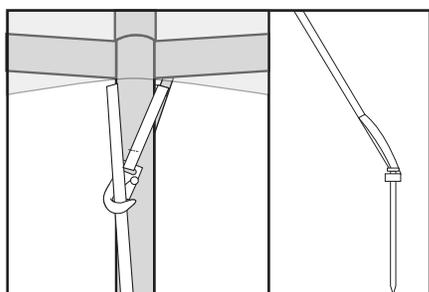
Locate the remaining 2 outguy straps. Connect the hook at the top of the strap to the intermediate bracket by looping the hook around the bracket and clipping it back on itself. Locate the 3' ground stakes and wrap the looped strap (found at the bottom end of the outguy straps) around the head of the stake twice. Drive the stakes into the ground 5' out from each corner leg and ratchet the strap until it is taut. Repeat this step on the 1 remaining intermediate leg.
