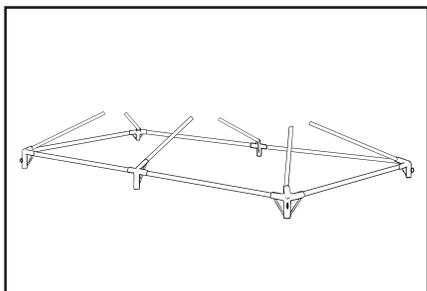
Insert hip poles into corner brackets at all four corners and ensure that the snap pins lock into place. Insert the intermediate poles into the intermediate brackets at both center points. All six poles should be installed with the open hole end towards the sky and the snap pin ends towards the ground. Ensure that all snap pins lock into place in all brackets.
