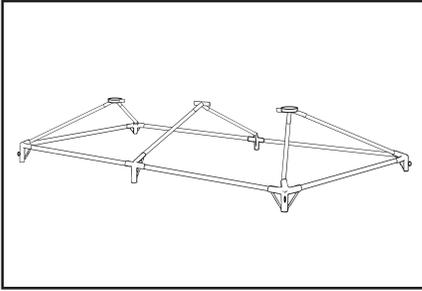
Install the crown cluster bracket by inserting both hip poles into the bracket. Repeat this step to install the second crown cluster. Once both crown cluster brackets are installed, put the roof rafter bracket into place by slipping it over the two intermediate poles - located in the middle of the setup.
