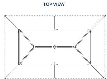
36" Stake driven within 6" from the top of the ground straight down or a maximum 10 degree angle
