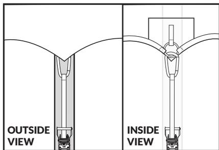
Locate the intermediate poles on the 20' sides of the tent. On the valance, where it comes down to a point and meets the pole, a single metal ring is sewn onto the inside of the tent top. Attach the carabiner at the top of the intermediate tent top strap to this metal ring.
