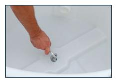
Connect the bottom carabiner on the outguy strap to the metal loop that is located on the bottom of the inside of the water barrel. Be sure that the remainder of the strap is outside of the barrel before moving on to the next step.
