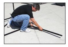
Insert a 4' - B pole into the bottom of the top corner bracket. Repeat for both the left & right sides.
