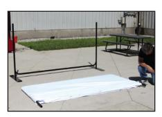
Slip this cover over the top pole section, leaving 6" of the left & right 4' poles exposed.
