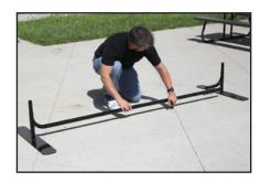
Insert the bottom pole section into both the left and right bottom corner brackets.
