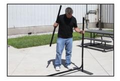
Insert a 4'- A pole into the top of the bottom corner bracket. Repeat for both the left & right sides.
