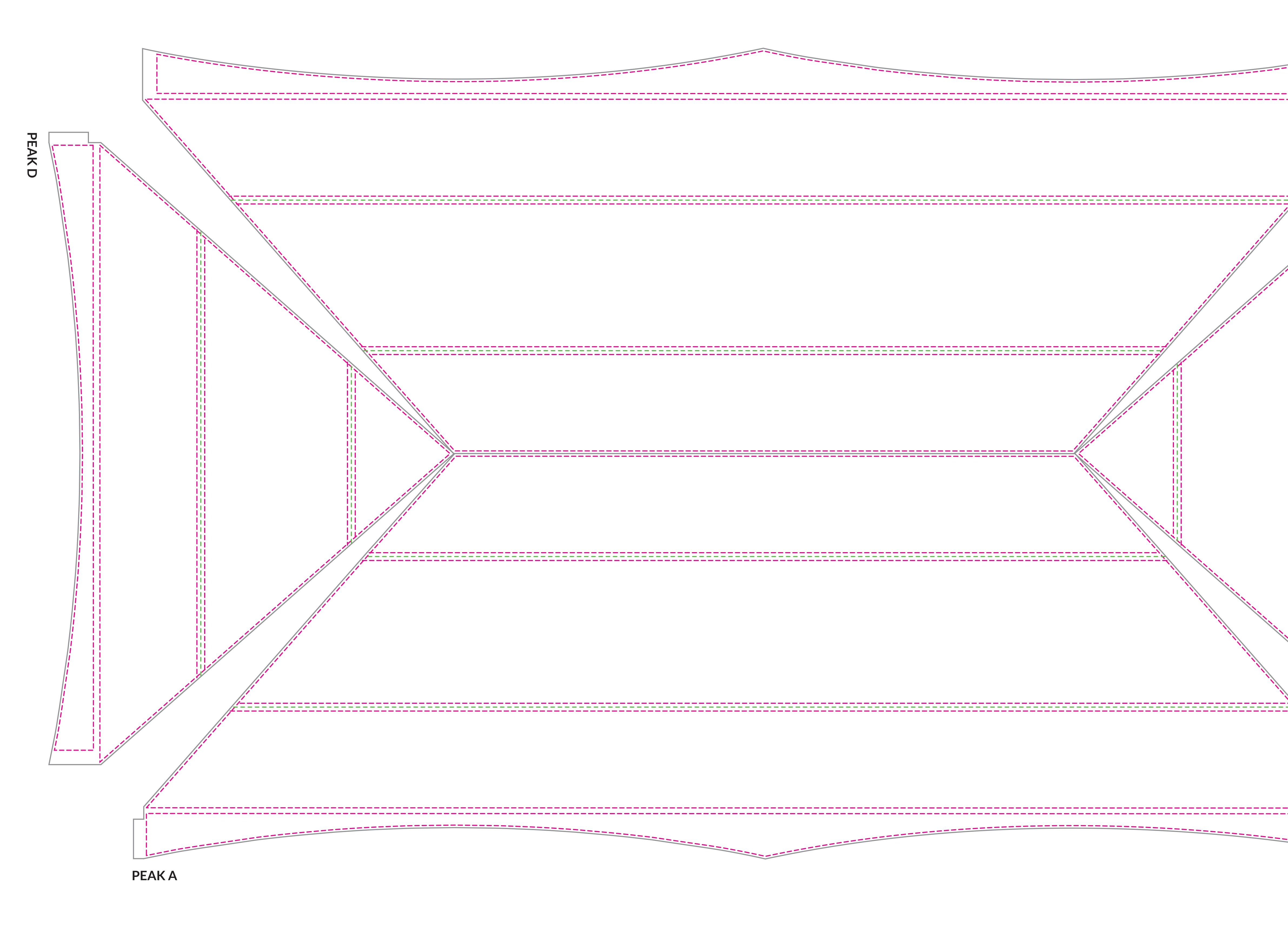
X-SERIES 20x40 ROOF - DECAL / PRINTABLE THERMAL / WHITE INK VISUAL: A/C 156.2"h x 482.6"w B/D 156"h x 243.6"w PEAK SAFETY: A/C 135.5"h x 476.6"w B/D 134.9"h x 237.6"w VALANCE SAFETY: A/C 16.5"h x 472"w B/D 15.9"h x 233"w
