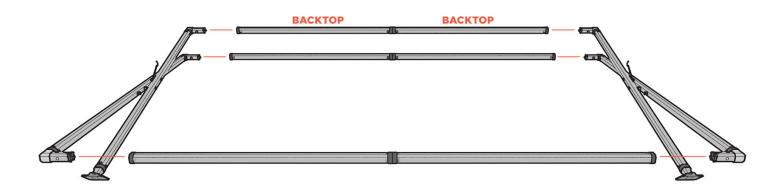
Grab the laser etched "BACK TOP" bar and connect it to the elbow brackets. (The opposite side of this piece ends in footpads.) Connect it by inserting the pole over the smaller, corner pole piece until it clicks in place.
