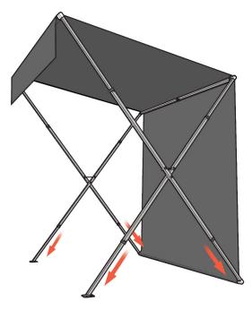
Extend the bottom 4 legs of each X. To extend, press the button and pull out the pole until it locks, extended, in place. Repeat for the remaining legs.
