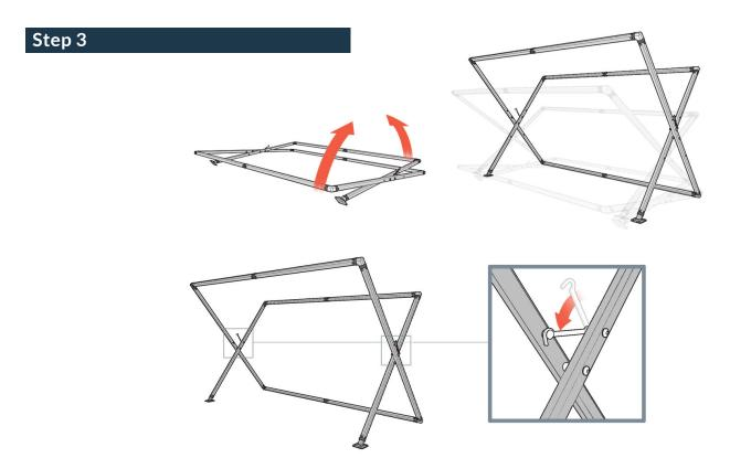
Lift up the top "X" frame pieces and latch the steel stabilizer hook over the catch on the opposite pole. This locks the "X" in place.
