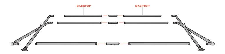
To start, lay out all parts on the ground in front of you as shown. Find the two back poles that are laseretched with "BACK TOP" and connect them together until the button securely clicks in place. Connect the remaining poles together the same way.
