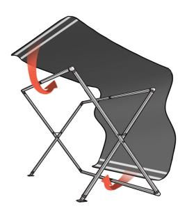
Drape the roof over the top of the frame.
