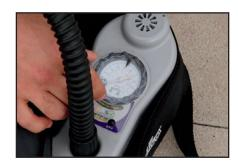
Locate the pump/battery pack and unzip the top. Insert the hose into the pump and set the dial to 41 KPA or 6 PSI (depending on the pump).
